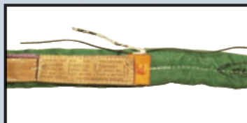
TATTLE TAIL MISSING (Sling fails inspection)
