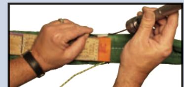
FIBER OPTIC-No Light Transfer (Sling fails inspection)
